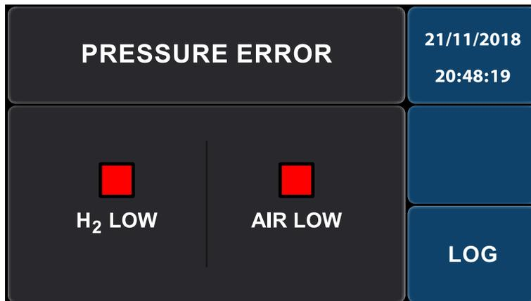
Low air & low Hydrogen pressure alarm - Figure 23
